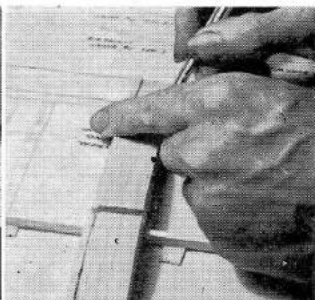
9 The positions of the trailing edges were marked on the ribs before separating them.
